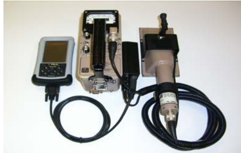
TDS Recon PDA, and Receiver with Electronics box (attached to Ludlum 2360 and detector)
